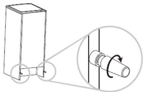
The appliance is supplied with two plastic spacers(in the plastic bag) of user manual). After installation of these spacers, the appliance cannot be pushed against the wall to maintain proper ventilation. Insert the spacers into the relevant openings on the back of the appliance, then screw the spacers tightly.
